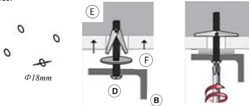
Step4: Tighten the screws .
