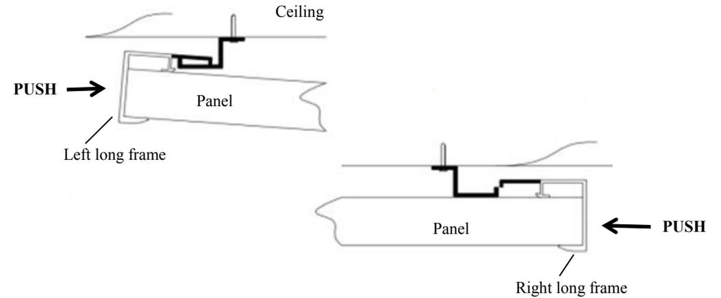
2. To avoid falling off, you must slide the panel left and right to make sure the two hooks have been completely put into the rear of the two long frames!
